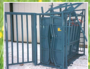
Bison chute with manual headgate
