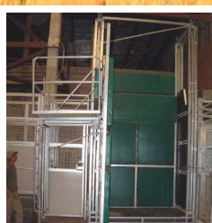
Emergency side exit opens full length of restraint to allow unrestricted release of animal. Picture above shows 3" padding on both sides.
