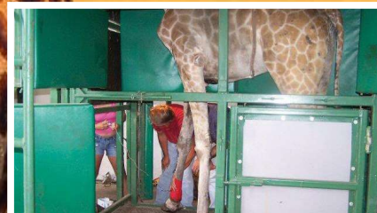
FIGURE 2 Eighteen different access doors to reach all areas on both sides of the animal.
